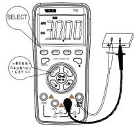
c) range has been exceeded and it is necessary to select higher range mode to complete this measurement.
