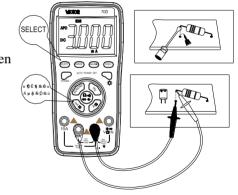
2. In case "OL" is displayed on the display, it indicates the current being measured has exceed the current
