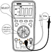
b)At automatic identification and measurement, the AC threshold voltage is 0.5V; in case the voltage to be measured is smaller than 0.5V;trigger the "SELECT" button to select automatic ACV measurement. In case the AC mV mode is used, please select the "RANGE" button.
