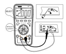
AC/DC current measurements, and if the current is lower than 10% of the range, the automatic identification is lower than its threshold, measurements cannot be conducted. Please press "SELECT button to select automatic range AC/DC current measurement.
